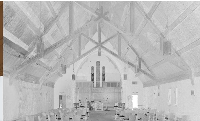
Church - Point Cloud to Revit
